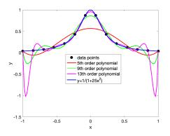
Notice that the approximation is getting worse at the endpoints as we increase the number of data. This is called Runge phenomenon and unfortunately it can happen in situations where data is collected on an equally spaced grid.
