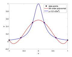
We see that the 5th degree interpolating polynomial does a particularly poor job of interpolating at the peak and near the endpoints of the interval. Lets try to increase the accuracy by adding more data points and letting n = 10.
